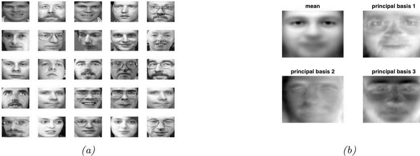
Figure 20.3: a) Some randomly chosen 64 \times 64 pixel images from the Olivetti face database. (b) The mean and the first three PCA components represented as images. Generated by code.probl.ai/book1/20.3 .
